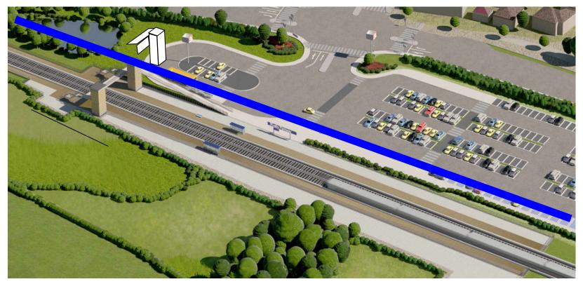
For example, while no substantial structures are shown in the illustration, if there are any substantial structures it would be prudent to locate them sufficient distance north of the existing tracks to allow an additional 5m wide single track to be accommodated (as indicated in blue).
