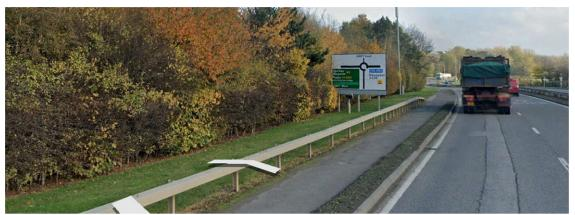
100m further along the road, again armco barrier appears to be protecting street furniture from collision, no protection provided for active travellers, who would be caught between motor vehicle and armco barrier if a motor vehicle mounted the pavement at this location.
