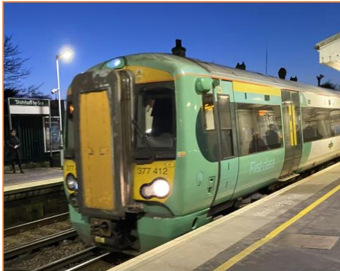
A Class 377 unit on a London Victoria train at Shoreham-by-Sea. These are of the Bombardier 'Electrostar' family of rolling stock.
